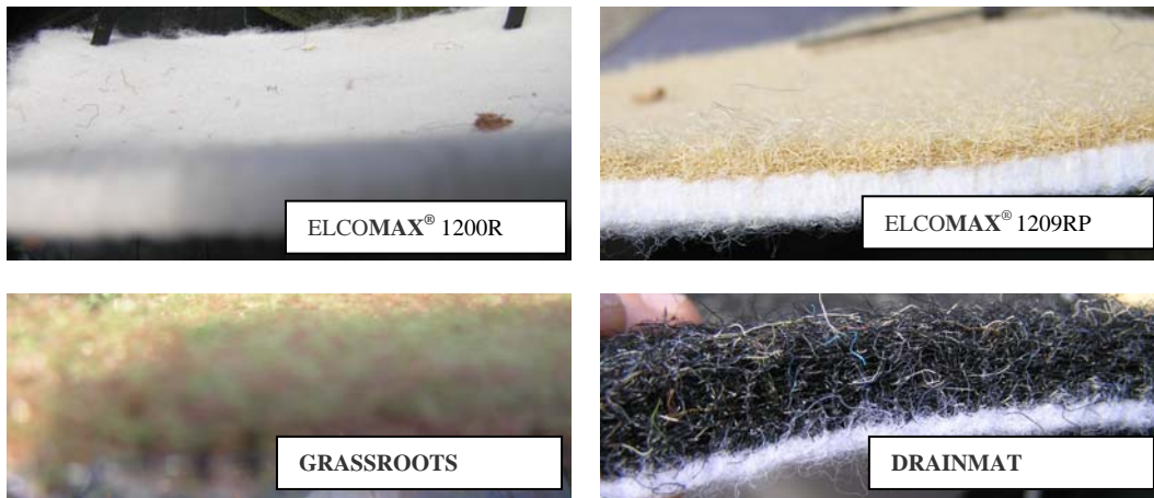
Figure 4. Geosynthetic 300mm square samples (ELCOMAX 1200R, ELCOMAX 1209RP, Grassroots, Drainmat)
