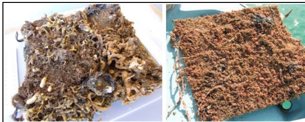
Figure 9. ELCOMAX 1009RP after (a) 3 years, Gold Coast and (b) 4 months, UAE
